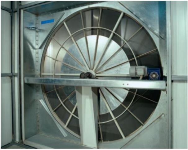
The automatic Rotary Pre-Filter Unit is ideal as a preliminary filtration stage of larger air streams, heavily charged with waste, coming from the production machines. It is a part of the proven compact centralized air handling system TexPac and optimally combinable with several function modules. This unit captivates by its simple and space-saving design and its reliable functionality.
