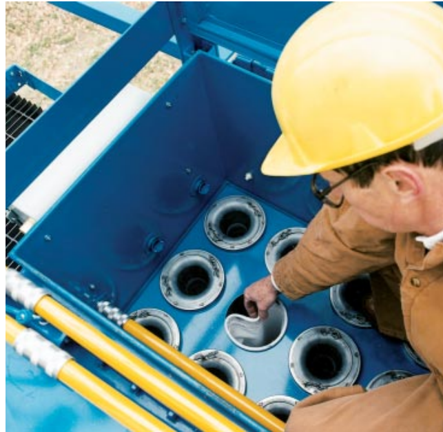
Snap ring filter bags and pulse pipes are removed and installed without tools on the STJ and CTR models.
