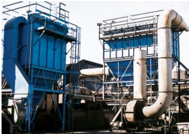
Two TubeJet collectors handle carbide dust and blast machine dust at this manufacturer. Unit at left handles 20,000 CFM; at right 60,000 CFM.
