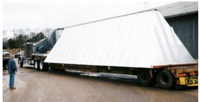
We can handle the big jobs, too! This 35,000 CFM TubeJet collector was shipped in three sections: walk-in plenum, filter housing, and trough hopper.
