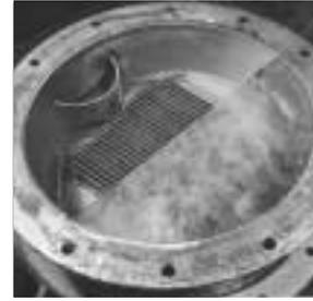
*Venturi Effect results in turbulent interaction of liquid and particulate-laden gas flowing through perforated plate and striking the wetted impingement baffle grid. (Each hole has an individual impingement surface.) Minute liquid droplets are formed which entrap suspended matter in gas. Particulate carrying droplets mix with water flowing across baffles for ultimate disposal through the drain. Cleaned gas passes through the mist eliminator for return to process or atmosphere.*
