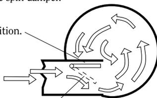
**Variable Spin Damper** is manually adjusted to control spin velocity. Proper adjustment maintains the spin velocity necessary to efficiently collect entrained liquid droplets.
