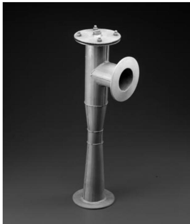
***Eductor scrubbers are designed to remove soluble gases and particulate by inducing a gas flow using high pressure liquid focused into a venturi throat. Additionally, eductor scrubbers can be used for direct-contact condensation. A high liquid flow rate makes the Sly eductor particularly appropriate for collection of sticky and/or gummy particulate, as well as gases which decompose upon contact with water, such as SiCl<sub>4</sub> and H<sub>2</sub>SiF<sub>6</sub>.***
