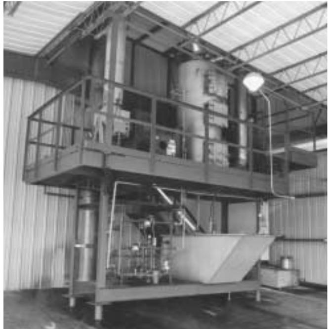
**Scrubber Cleans and Absorbs Acid Gases and Particulate From Medical Waste Incinerator** — An Impinjet® wet gas scrubber is used by this company to clean exhaust gases from its medical waste incinerator.
